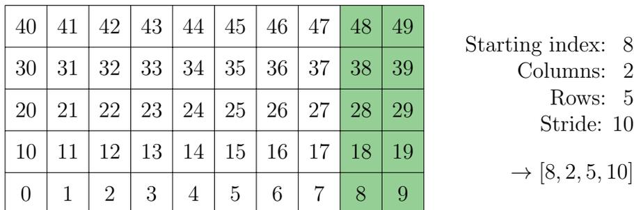
Figure 2.2: Example of compressed storage: 10 integers (40 bytes) stored using 4 integers (16 bytes), halo region highlighted in green.
